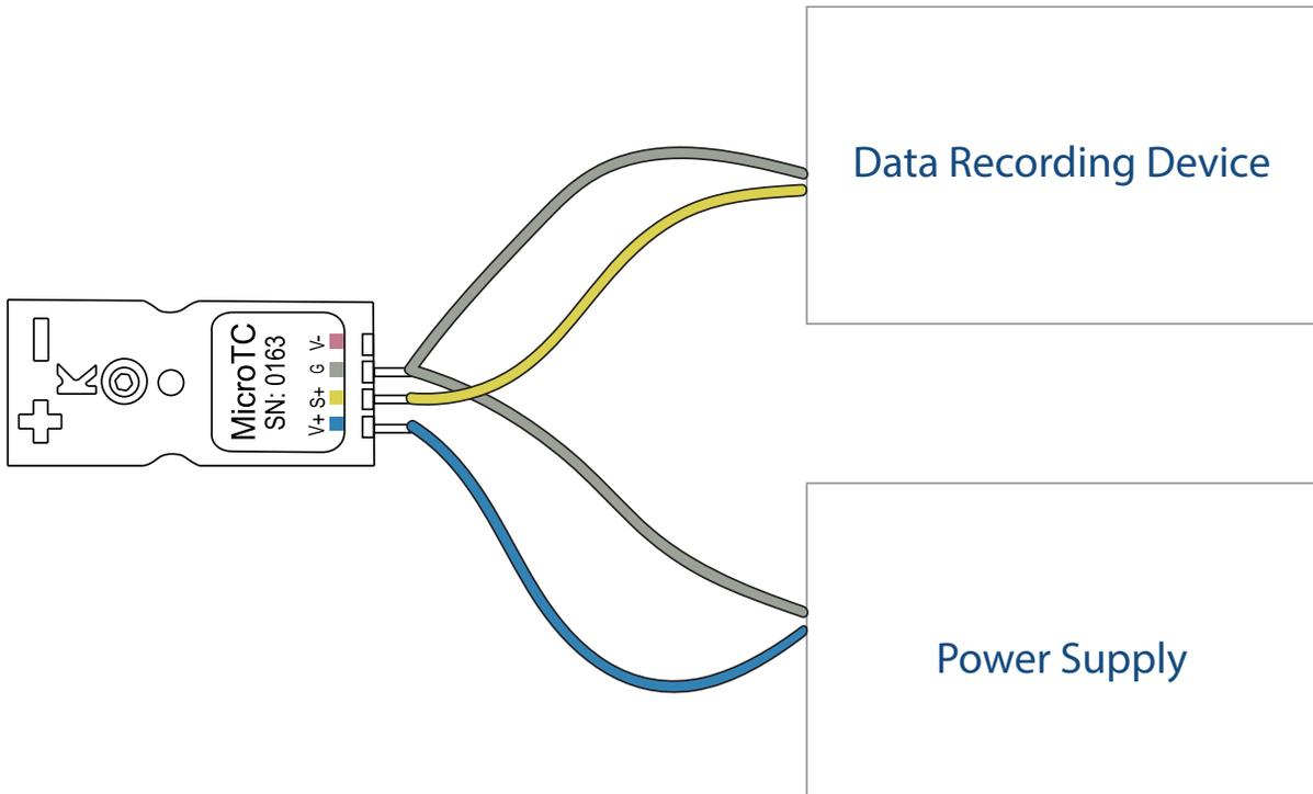
The output high is measured relative to the ground wire. It is recommended that a separate wire for signal common is added to the common terminal to reduce errors from voltage drops along the power common wire. When using the MicroTC with a slip ring assembly, a separate signal common can be added to the stator of a slip ring to decrease the amount of rings needed, but it is important to place the amplifier as close as possible to the slip ring.
