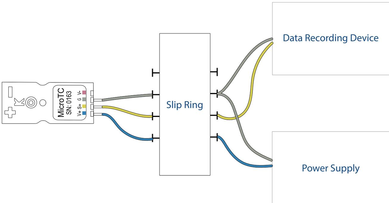
The thermocouple sensor should be attached using the provided mating connector (Omega± HMPW-\*-M). If a thermocouple input is left unused or if the thermocouple opens, the output of the amplifier will rise to V+. The amplifier will not be damaged if a thermocouple is left unattached.
